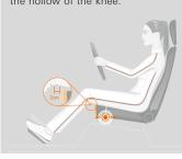
as possible on the backrest. Set the backrest tilt so that the steering wheel is easy to reach with slightly bent elbows. Shoulder contact must be maintained when the steering wheel is turned.
