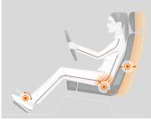
5. Adjust the extendable seat cushion so that the thighs rest on it to just above the knee. Rule of thumb: two to three fingers Space between the edge of the seat and the hollow of the knee.
