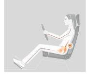
3. Set the seat height as high as possible. This ensures an unobstructed view to all sides and all displays on the instrument
