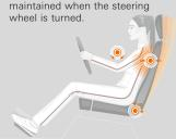
6. The lumbar support has been adjusted correctly when the lumbar part of the back is supported in its natural shape.
