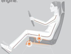
**5.** Adjust the extendable seat cushion so that the thighs rest on it to just above the knee. Rule of thumb: two to three fingers Space between the edge of the seat and the hollow of the knee.
