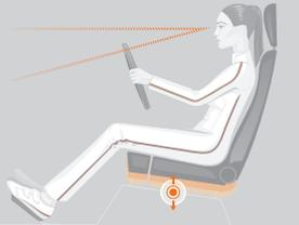
**4.** Set the seat cushion tilt so that it is easy to depress the pedals fully. The thighs should rest gently on the seat cushion without exerting pressure on it. Check the backrest tilt before starting the engine.
