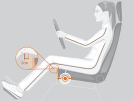
**6.** The lumbar support has been adjusted correctly when the lumbar part of the back is supported in its natural shape.
